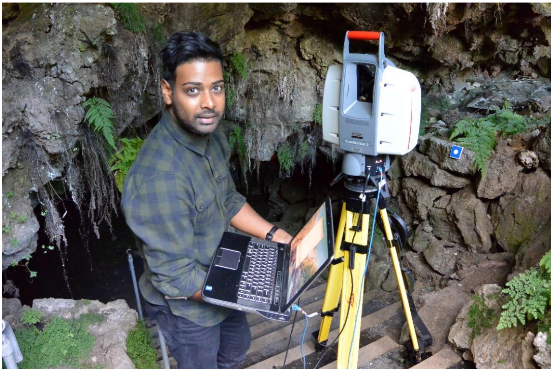
Figure 3. Chirag Jindal with his 3D Lidar, or Laser scanning equipment, which is used to capture data that is used to produce highly accurate and detailed 3D cave maps.
