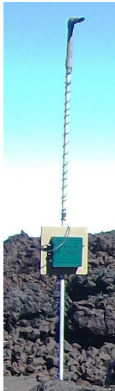
Figure 4. An acoustic recording station with SM2Bat recording unit (green box) attached to a galvanized steel pole. An extension cable connected to a high frequency microphone is wrapped around the pole to secure it from high winds.
