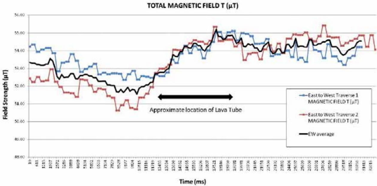
Figure 2 - Total Magnetic Field on East to West Traverse Line above Raufarhólshellir
