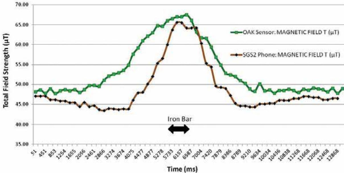
Figure 8 - Direct Comparison of Phone with External Digital Magnetometer
