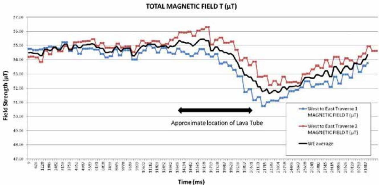
Figure 3 - Total Magnetic Field on West to East Traverse Line above Raufarhólshellir
