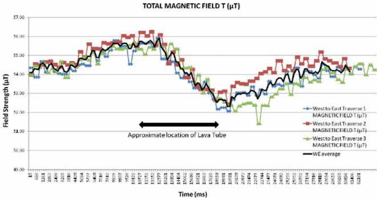
Figure 5 - Total Magnetic Field on West to East Traverse Line above Tagli
