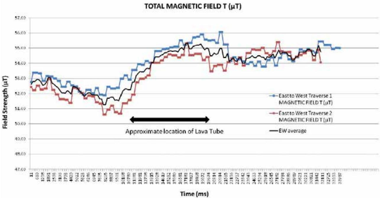
Figure 6 - Total Magnetic Field on East to West Traverse Line above Un-named Lava Tube
