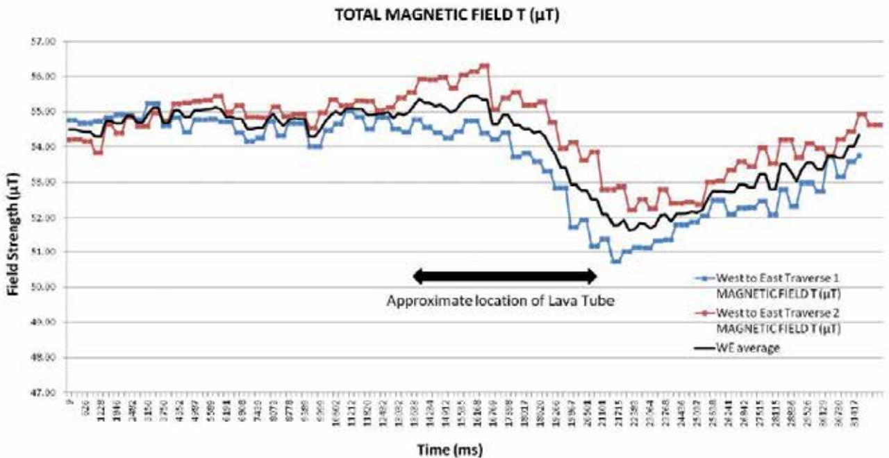
Figure 7 - Total Magnetic Field on West to East Traverse Line above Un-named Lava Tube
