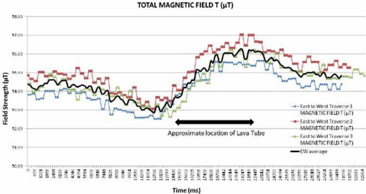
Figure 4 - Total Magnetic Field on East to West Traverse Line above Tagli
