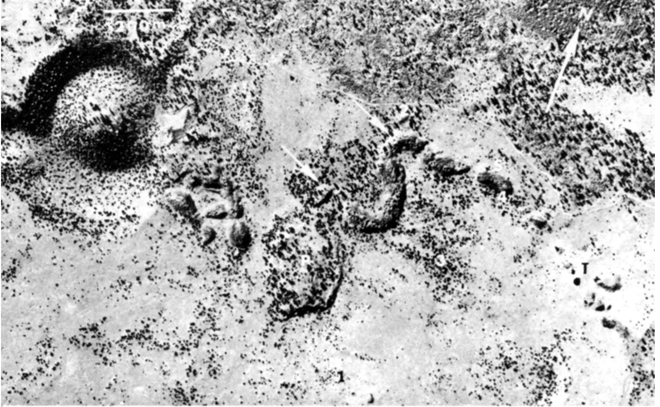
Figure 4-6: Sinuous bends along the lava tube issuing from El Calderon Crater. Four distinct tubes (1 thru 4) branch from the subsidence pit (P). Collapse of tube number 4 is evidenced by S (straight-sided collapse pits) and T (tensile failure producing a hole in the roof of the tube). (Ariz.fig.7-R)
